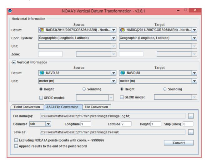
The geotags.txt file obtained from post processing can be converted with the settings in the image above.
