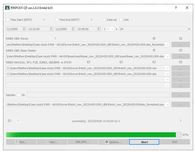
The processing bar at the bottom of the screen will go forward to 100% and backward to 0% to ensure the highest quality of data has been achieved. After processing has finished there will be a file with the ending events.pos containing the positions that the images were captured at.
